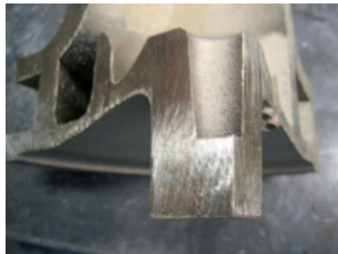
Hub with no shrink cracks present.
