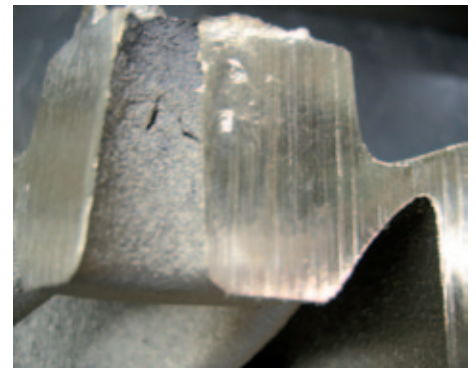
Original shrink defect found in the heavy hub section of the casting
