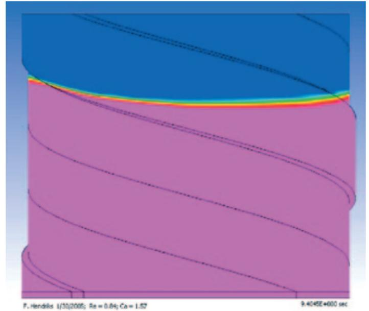
Figure 2. Computed average deflection of the oil air interface in the 1000X scale up model under 1G gravity. 1 cell discretization across the oil film. The average interface deflection agrees well with the deflection of the scale up experiment.
