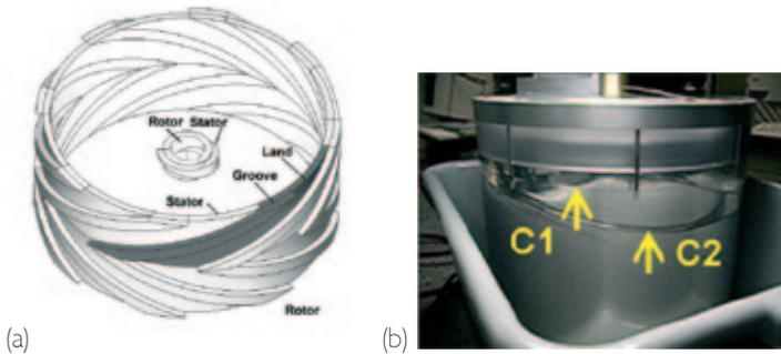
Figure 1. (a) Typical FDB herringbone bearing with 8 land/groove sections. To study a single land/groove pair shown in black, it was rolled up onto itself to form the tiny object at the center.
