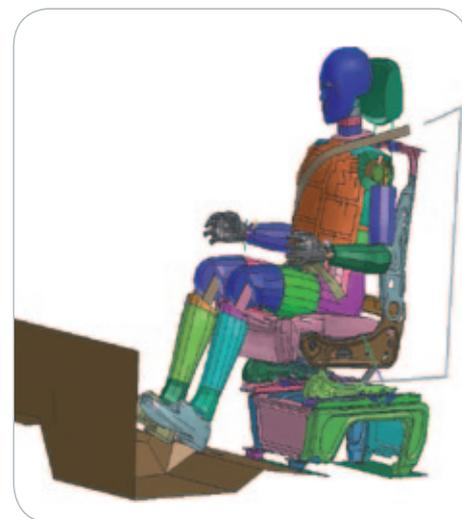
Sled test with a Hybrid III 50e percentile on a driver seat (AMS 50 km).
