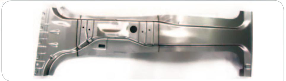
B-pillar stamped from tailored blank with 3 thicknesses and 2 weld lines (visible)
