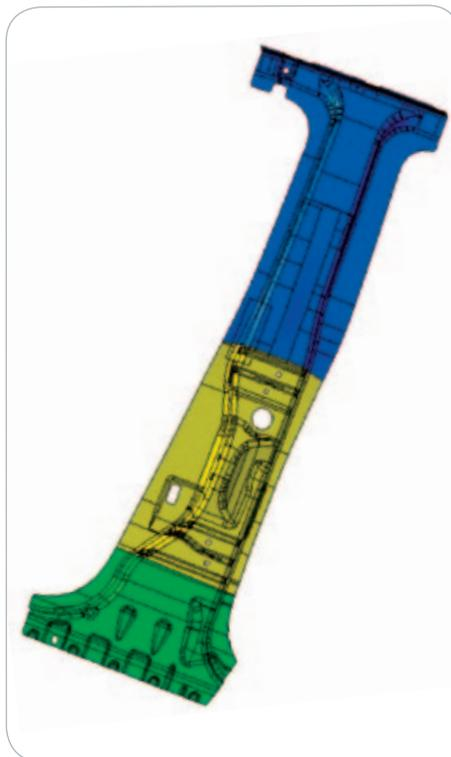
Transitions between different thicknesses must be seamless to reach required surface quality
