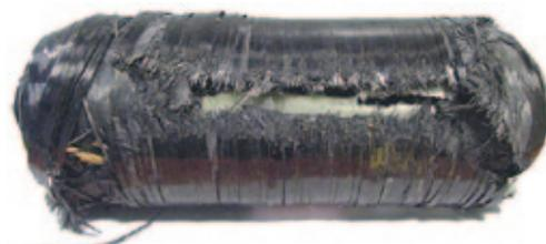
CEA 37L H2 high pressure vessel after burst test. Courtesy of the CEA.
