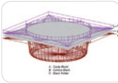
Representation of the mold, blank and blank holder.
