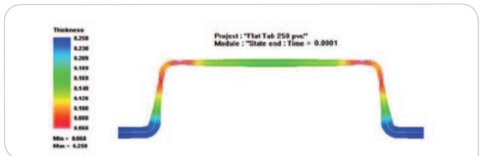
Simulated thickness distribution at various locations in a blister pocket.
