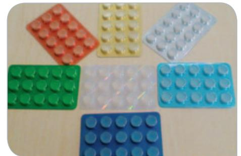
The different parameters like forming temperature, pressure/vacuum range, visco-elastic deformation properties of plastic material, die geometry, contact and friction between the blank and die, have a direct effect on wall thickness distribution in thermoformed blister. Thus, it is important to predict the wall thickness distribution on the blister cavity formation of the barrier films to determine the barrier property of the final blister pack.
