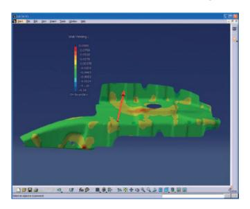
PAM-TFA for CATIA V5 provides a new workbench integrated into CATIA V5, offering state-of-the-art inverse simulation capabilities for metal forming applications directly within the CAA V5 environment.
