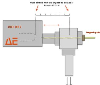
Figure m1: Schematic showing installation of translatable Langmuir probe within the remote plasma source and downstream tubulature
