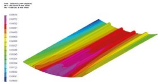
Detailed visualization of the normal displacement on a section of a stringer
