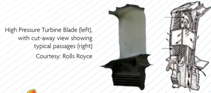
High Pressure Turbine Blade (left), with cut-away view showing typical passages (right)
