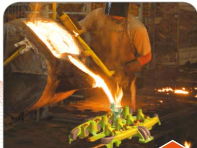
Filling of Cast Iron (Sand Casting).
