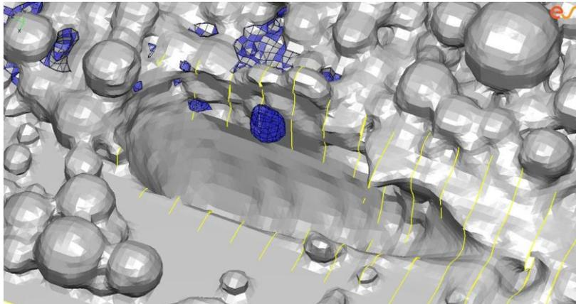
**Figure 4: Top view of the melt pool, where the upper surface is hidden. The melt pool shape and dimensions can be readily measured. The blue sphere shows a bubble that was captured in the melt pool and that is later captured on the solidifying material.**
