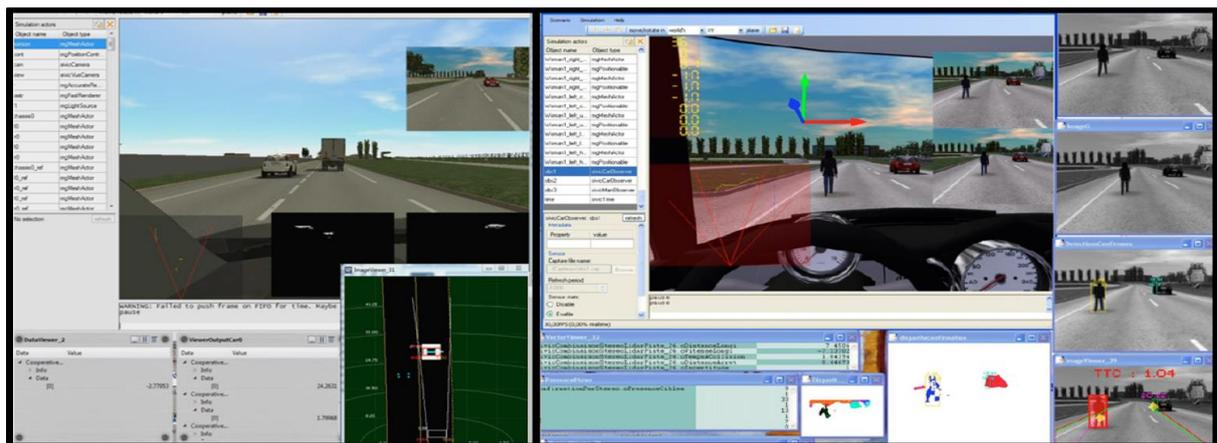
Figure 4: Examples of Pro-SiVIC use for virtual sensors and ADAS simulation
