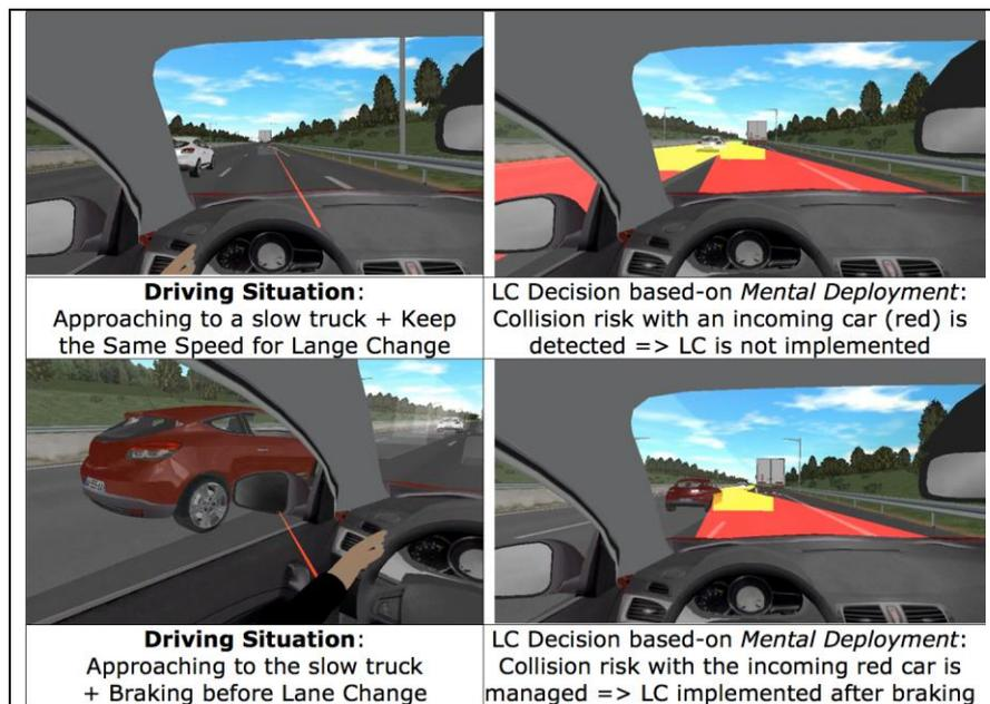
**Figure 2: simulation of decision making processes based on mental deployments**
