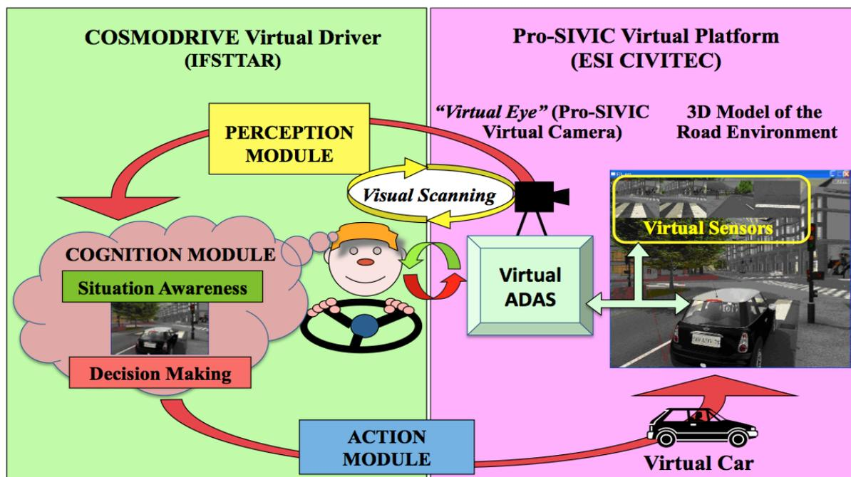
Figure 5: The V-HCD platform, interfacing COSMODRIVE and Pro-SIVIC
