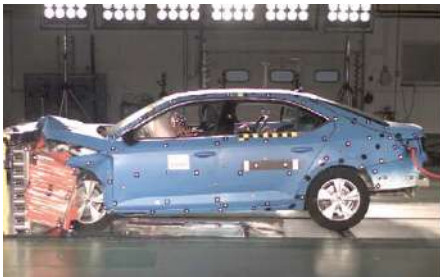
Physical test versus simulation of a frontal impact with ESI Virtual Performance Solution
