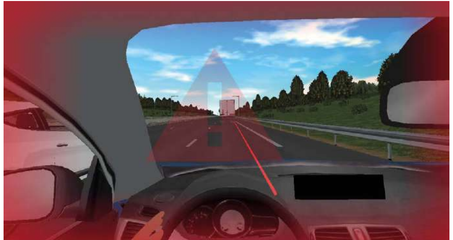
The cognitive model uses the simulated sensors' input to detect changes in the environment (slow truck ahead, passing car,...) and update situational awareness 1 .
