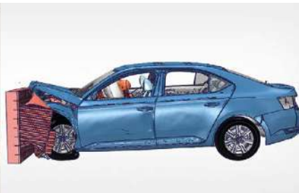
Physical test versus simulation of a frontal impact with ESI Virtual Performance Solution
