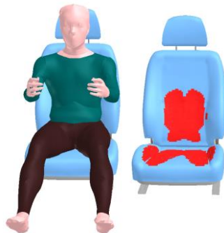
Figure 4. Seating of occupant and contact area Simulated with ESI Virtual Seat Solution
