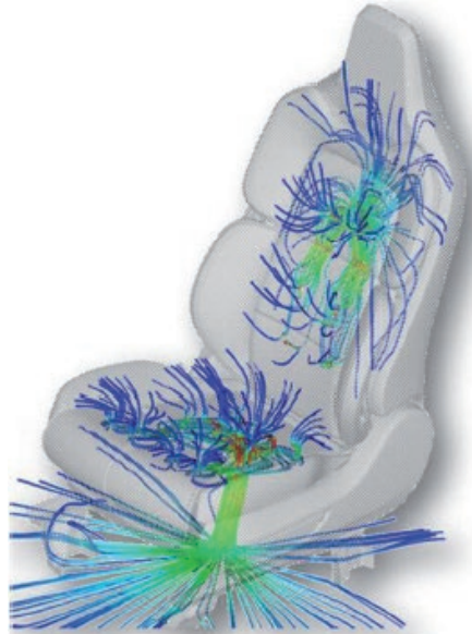
Ford engineers evaluated the performance of climate-controlled seats at ambient and extreme temperatures and predicted the impact on their lifecycle, using ESI Interior Solution. Image courtesy of Ford.
