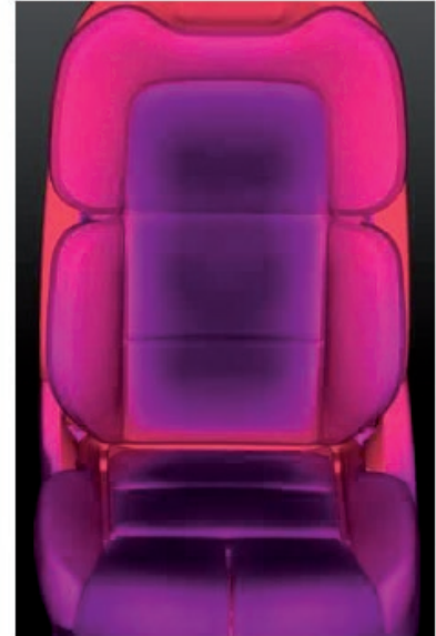
Ford engineers evaluated the performance of climate-controlled seats at ambient and extreme temperatures and predicted the impact on their lifecycle, using ESI Interior Solution. Image courtesy of Ford.
