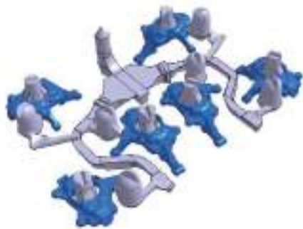
6-cavity die vs. Simulation Driven 8-cavity die
