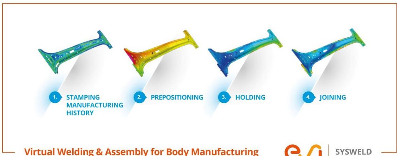
Image: Inheriting details of the “as manufactured” components from the press shop, ESI SYSWELD simulates the entire assembly and welding process chain in the body shop; step by step.
