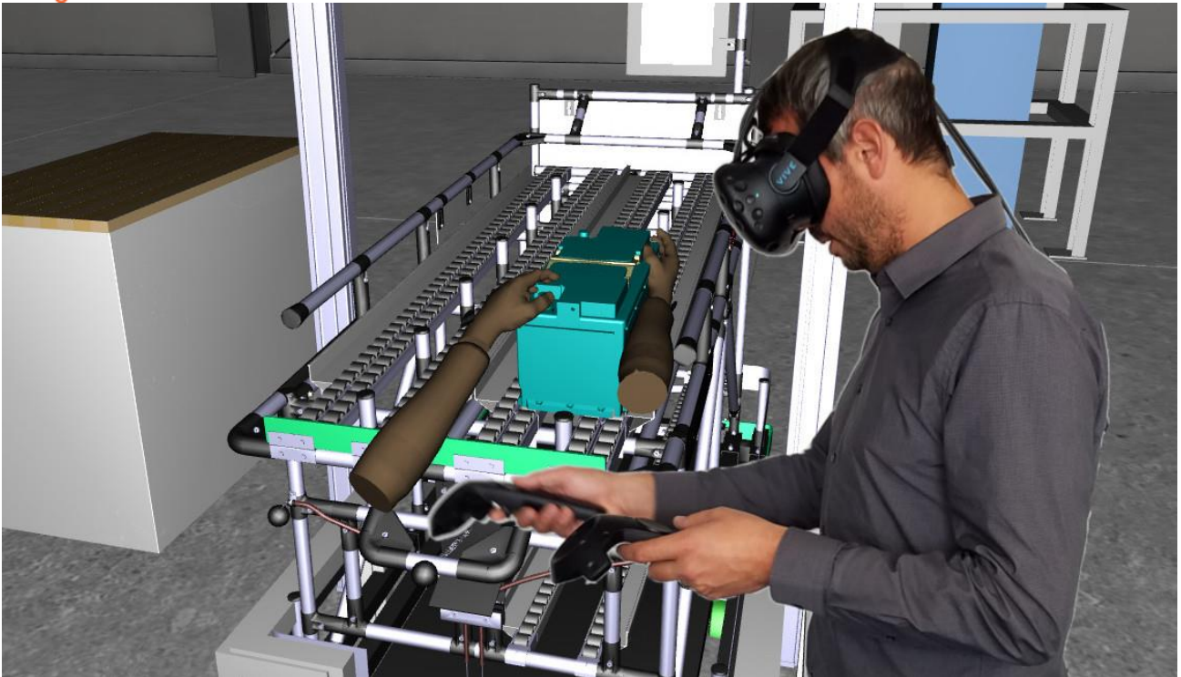
Image: Assembly process review conducted using ESI IC.IDO 11 with an HTC Vive Business Edition HMD.
