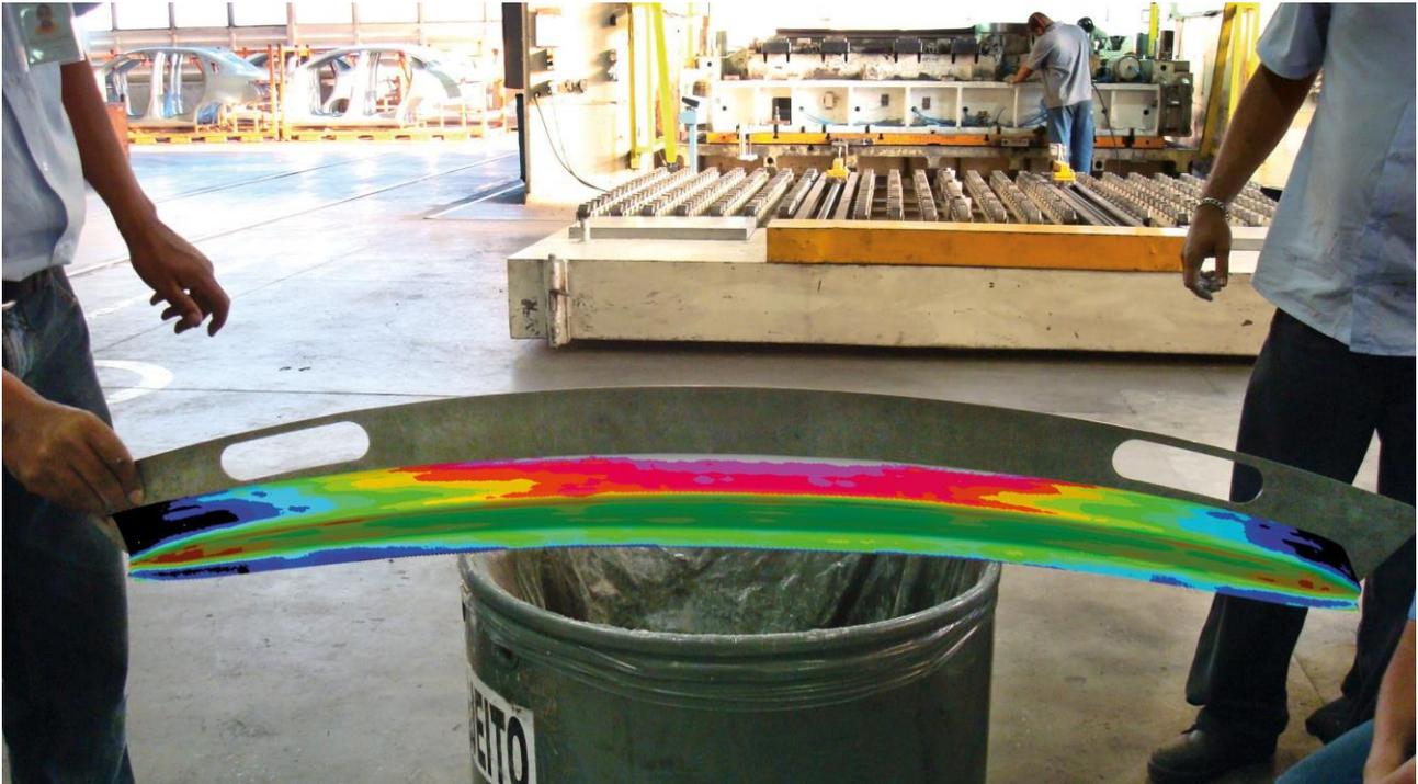
Image: From simulation to reality: thanks to ESI PAM-STAMP, customer Aethra manages to compensate significant springback effects. Read the full story [here](#).
