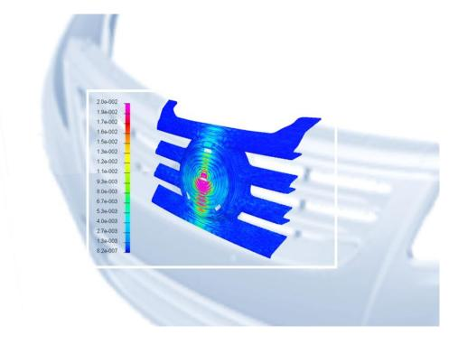
Image: RADAR sensor radiating across front plastic grill (Induced currents at 77 GHz)
