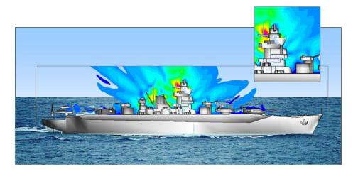
Near Radiated Fields of an Antenna on a Navy Cruiser
