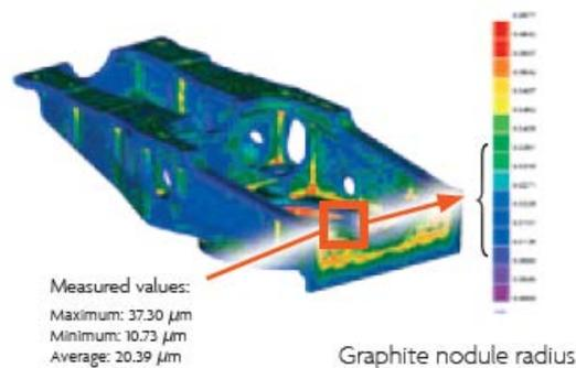
*Good correlation of the microstructure between simulation and real part.
