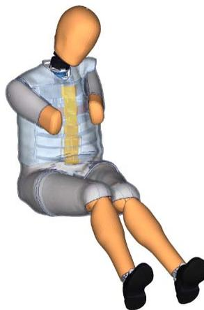
*World SID 50<sup>th</sup> dummy deformation mode under loading in a barrier test*
