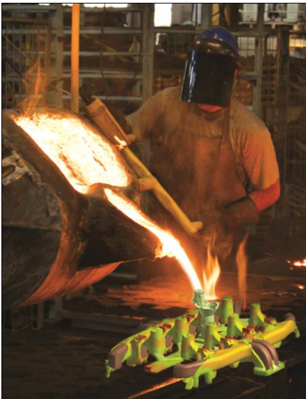
Filling of Cast Iron Sand Casting Courtesy of Fonderia Casati
