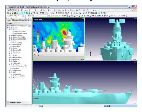
Electromagnetic radiation of a naval antenna (Visual Environment)
