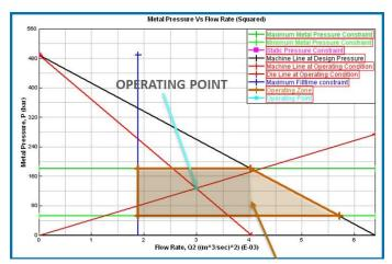
Image: Pressure(P)-Flow Rate(Q)<sup>2</sup> Graph, as seen in ESI ProCAST
