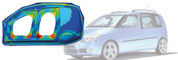
Stamping simulation of a car door. Courtesy of SKODA Auto.
