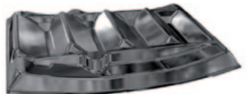
Original 23 piece welded design (top) and one-piece design optimized for SPF (bottom)
