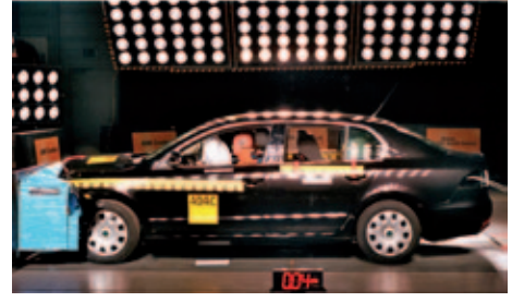
Škoda Superb frontal impact: 5 stars at EuroNCAP crash test certification Courtesy of SKODA AUTO
