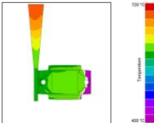
Figure 7: Temperature contours showing the position of the pyrolytic zone after 12.8 seconds (Procast™).
