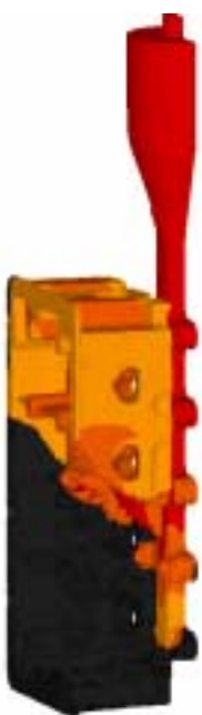
Figure 10: (left) Casting without the accelerator slot. Filling starts entering the casting through the top in-gates.
