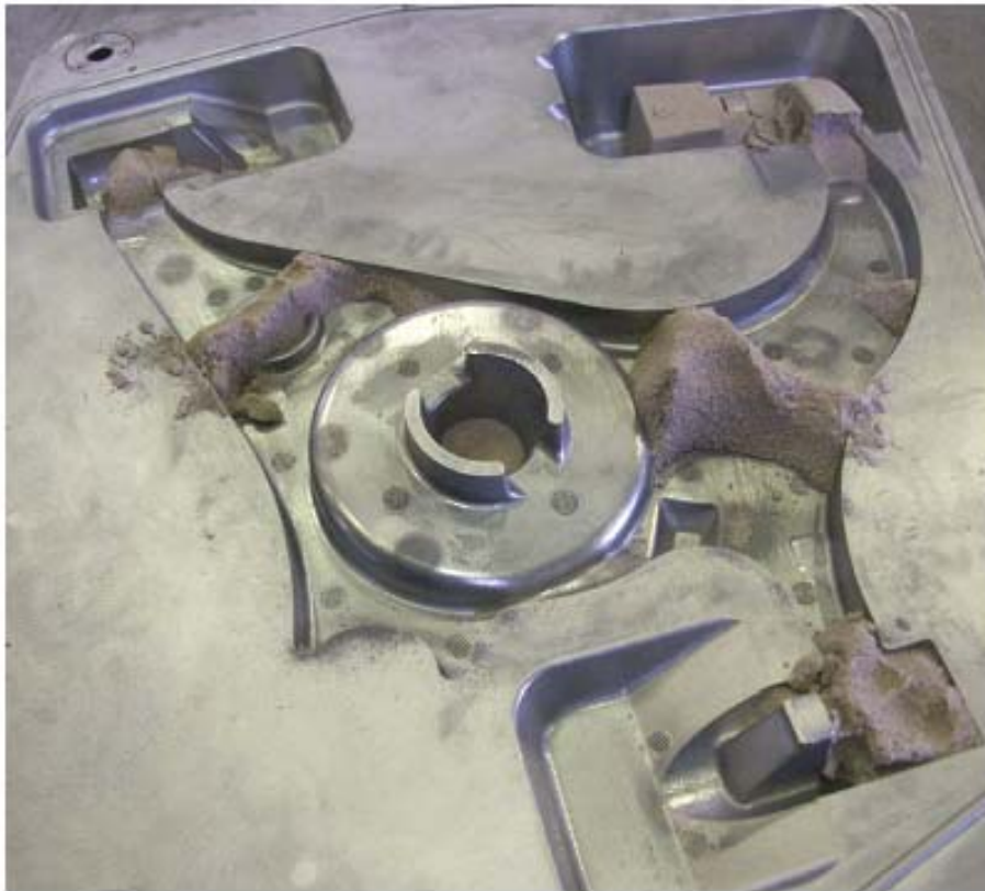
Figure 9: Remaining sand in the core box after an incomplete gassing process.
