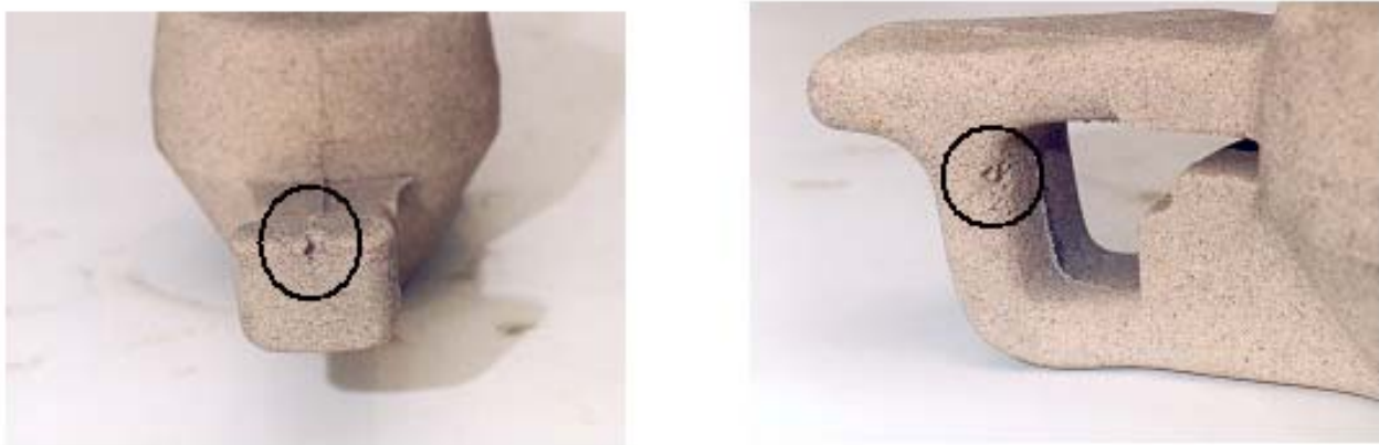
Figure 6: Unfilled areas observed on the axle core (courtesy of Infun).
