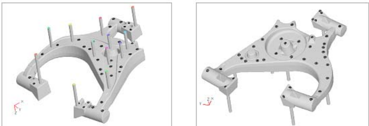
Figure 8: Suspension arm core geometry and vents positioning on upper and lower core box.
