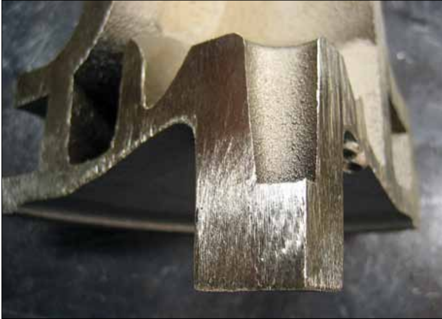
Prior to the use of Quikcast simulation, J. Walter Miller Co. used a closed riser and cored hub design, which produced a shrink pocket in the wear ring.
