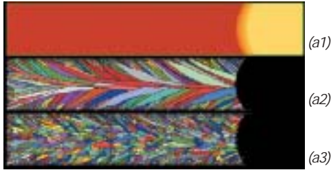
Figure 2: Solidification pattern at low casting speed (1mm/s). (a1) Solid / Liquid transition (solid = red; liquid = yellow). (a2) Grain structure without inoculation. (a3) Grain structure with inoculation. Structure predicted with the simulation software calcosoft®-2D.
