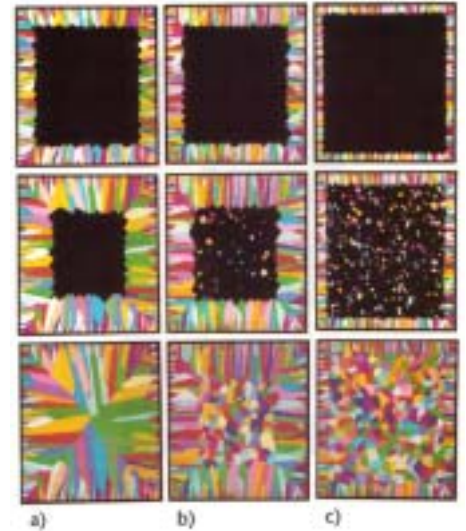
Figure 1: a) Purely columnar grain structure. b) Low inoculation, columnar-to-equiaxed transition. c) Strong inoculation, small columnar structure, mainly equiaxed grains. Grain structure predicted with the simulation software calcosoft®-2D.
