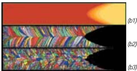
Figure 3: Solidification pattern at high casting speed (5mm/s). (b1) Solid / Liquid transition (solid = red; liquid = yellow). (b2) Grain structure without inoculation. (b3) Grain structure with inoculation. Structure predicted with the simulation software calcosoft®-2D.
