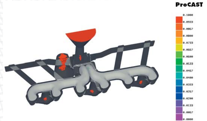
(c) when considering the graphite expansion with a high level of inoculation.
