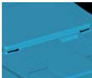
Simulation result of the crack, with element remove technology
