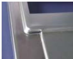
The crack of the left corner of the part (Actual photo)
