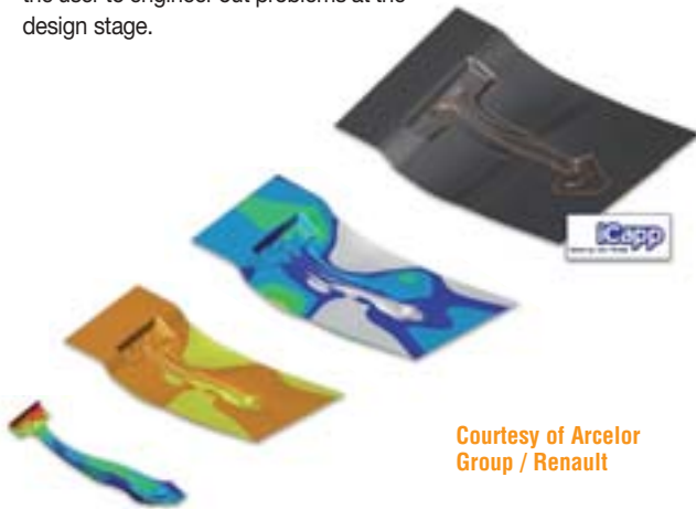
Fast and Accurate Automatic Springback Compensation with PAM-STAMP 2G
