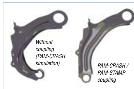
4 - Results of the steered wheel lateral pavement shock calculations
