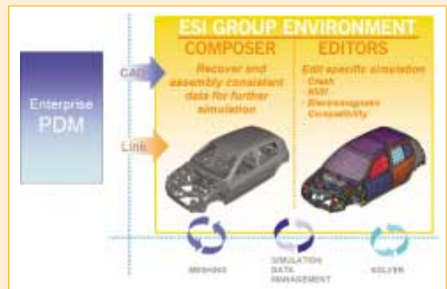
Renault group, early adopter of the COMPOSER application for Body-in-White finite element model generation and management
