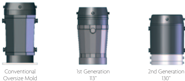
Fig 2: Mold design development
